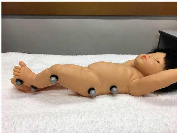
Figure 1 Marker placements for spontaneous kicking data collection.
