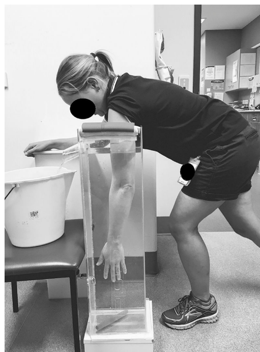
Figure 2 Volumetry tank with position taken by participants for measuring water displacement.
